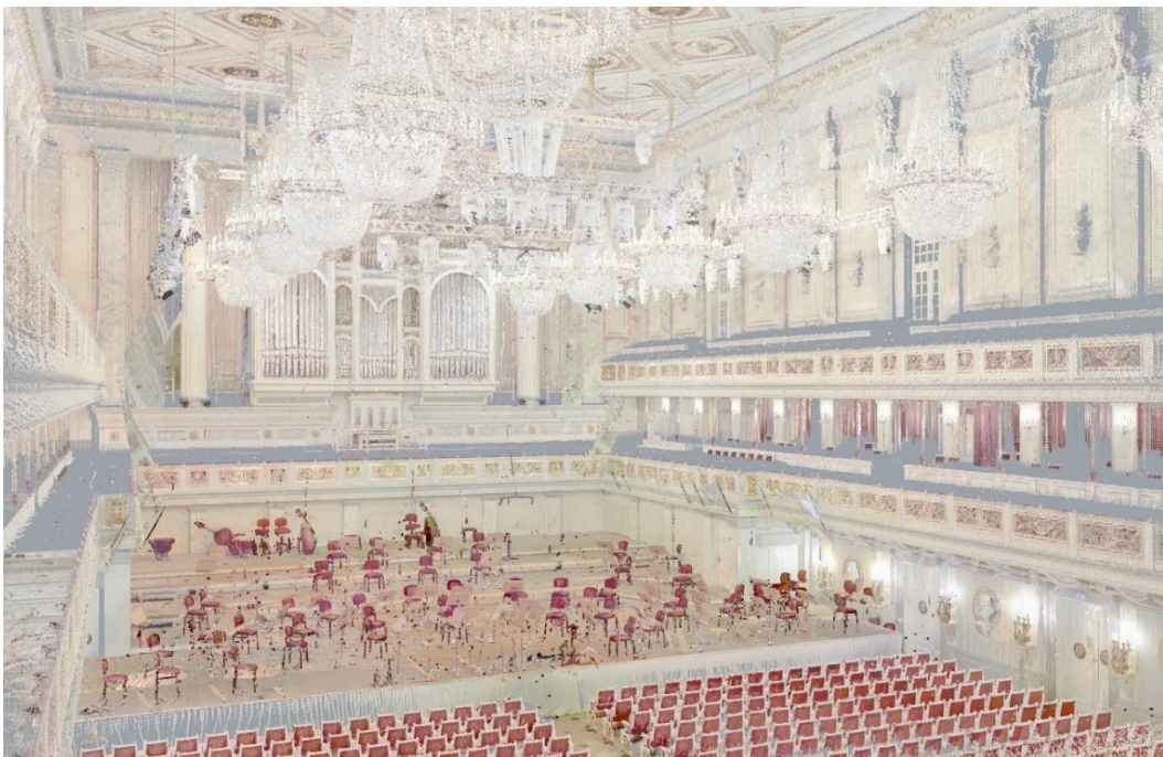
Decimated point cloud of the main hall inserted within the 3D modelling software
