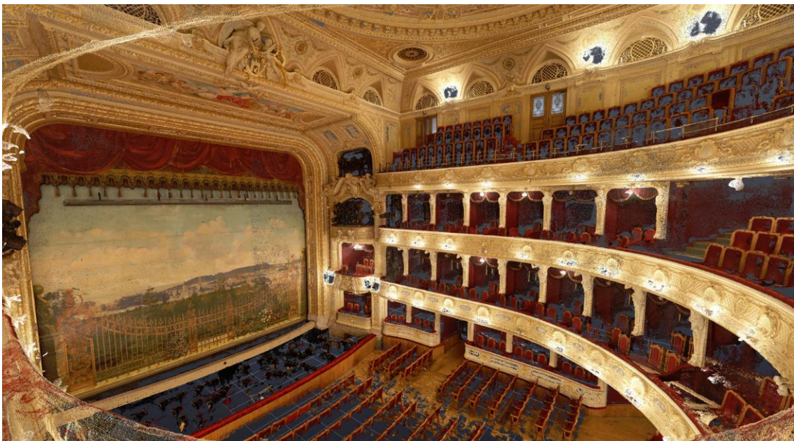
Coloured point cloud of the main hall processed through SfM photogrammetric methodology
