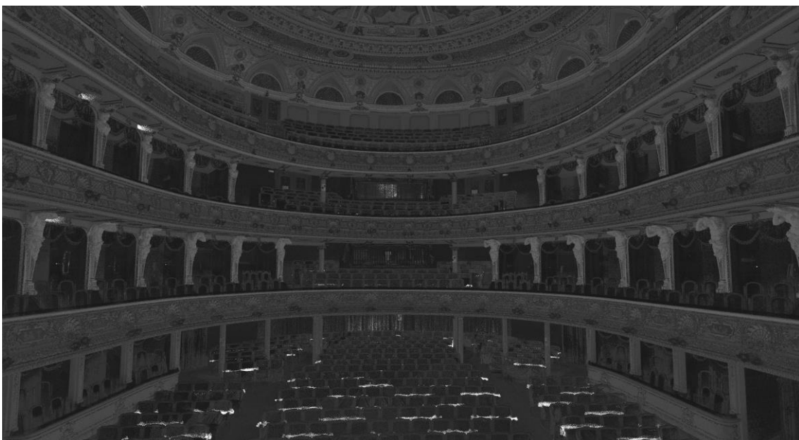
B/W point cloud of the main hall of the Lviv Opera House acquired and processed by the LPNU team
